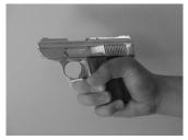
reveal that a round can be chambered with the magazine removed.
