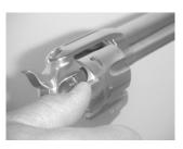
II Visually and physically inspect each chamber, to ensure that the revolver is unloaded.
