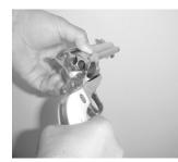
III Remove the firearm safety device required to be sold with the handgun. If the firearm safety device prevents any of the previous steps, remove the firearm safety device during the appropriate step.
