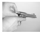
V. Open the loading gate and unload the revolver.
