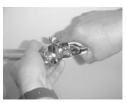
VI Visually and physically inspect each chamber to ensure that the revolver is unloaded.
