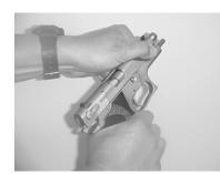
X Lock the slide back to eject the dummy round. If the handgun is of a model that does not allow the slide to be locked back, pull the slide back and physically check the chamber to ensure that the chamber is clear.
