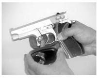
V Load one dummy round into the magazine.
